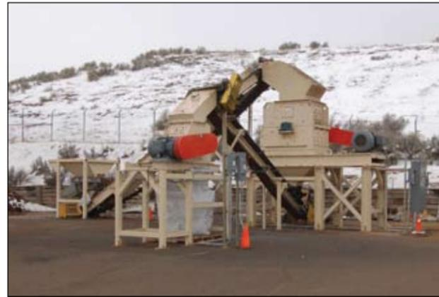
*This hammer mill is designed to crush cast-iron dummy bombs into a medium suitable for use in Permeable Reactive Barriers.*
